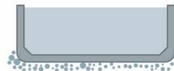
Computerised image of air bubbles under a vessel's hull
