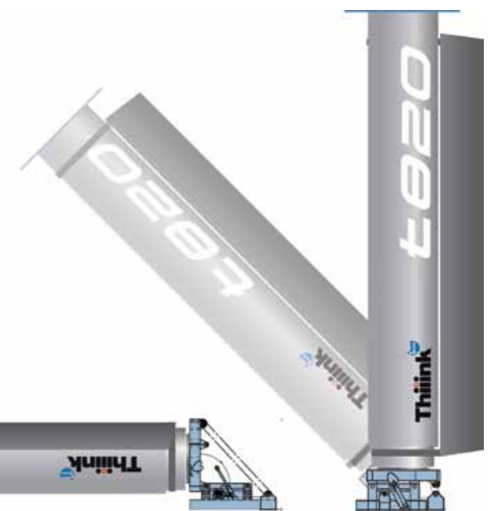
Computer-generated image of Thiiink's Flettner rotors
